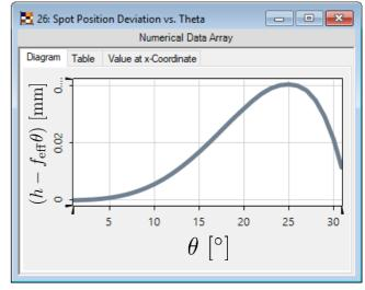
analysis of deviation between actual and the desired focal spot position
