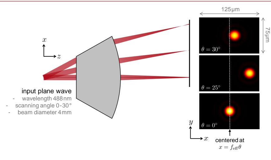
Deviation between actual and the desired focal spot position indicates the performance of the F-Theta lens.
